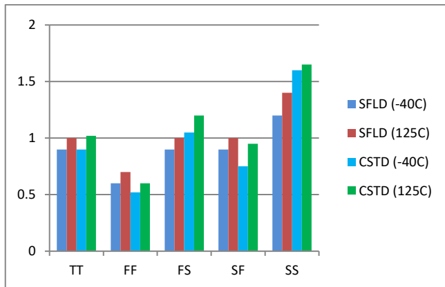
Fig. 10 Corner analysis for proposed circuit CSTD with SFLD at varying temperature and front end process corners on normalized delay of the circuit.
